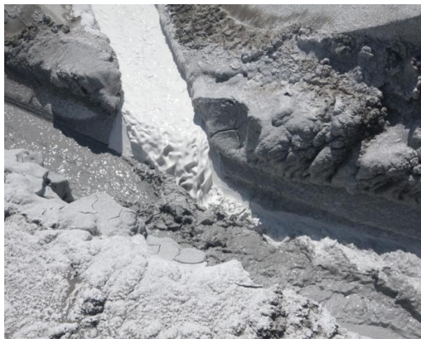
Figure 15: Thickener from blowdown (left stream) and underflow sulfate/sulfite solution (right).
