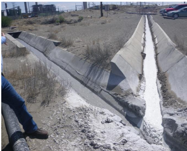
Figure 15: Thickener from blowdown (left stream) and underflow sulfate/sulfite solution (right).
